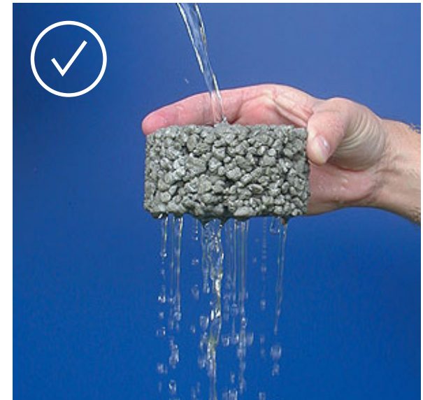
Porous concrete allows water to filter into the ground.
